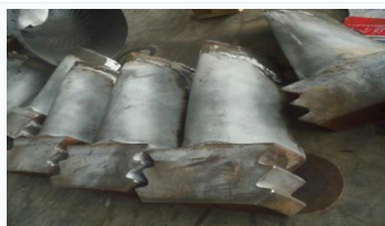
Bucket Repair 动叶片修复
