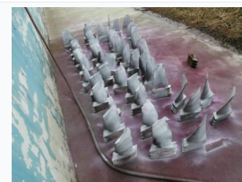
Moving Blade NDT 动叶片无损检测
