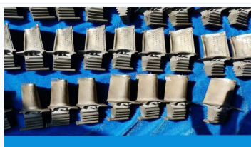
GE LM2500 1st-stage Turbine Blade (Single-Crystal Blade)
