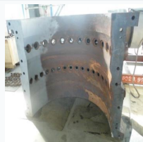
Casing Damage 缸体损伤
