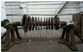
Rotor Bending Straightening
