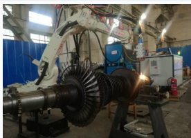
Laser Cladding on Damaged Rotors / Dynamic Balancing / NDT
