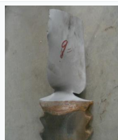
Bucket Damage 动叶片损伤
