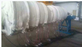
Rotor Bending Straightening
