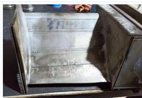
Mitsubishi Gas Turbine 1st-stage Guide Nozzle Before and after repair
