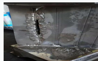
Mitsubishi Gas Turbine 1st-stage Guide Nozzle Before and after repair
